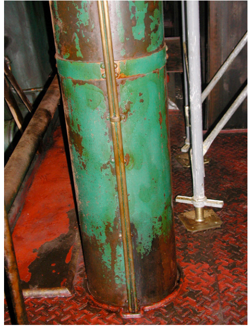
Figure B2. Originally painted surface, Worthington engine after treatment.
