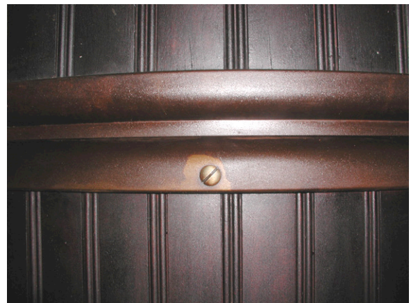
Figure C2. Originally plated surface, Leavitt engine after treatment.
