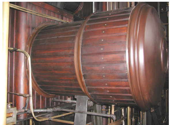
Figure M2. Finished wood elements at Leavitt engine after treatment.
