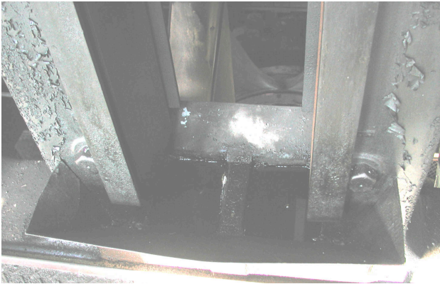
Figure K1. Standing oil build-up at Allis engine before treatment.
